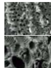
Electron micrographs of activated carbon pores
