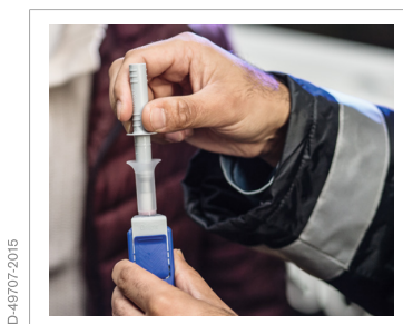
2. Insert the sampler into the funnel opening
