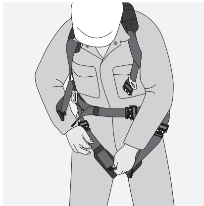
Tighten straps and retain free webbing within the elastic webbing tidy
