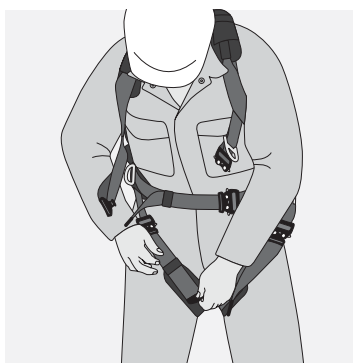
Tighten straps and retain free webbing within the elastic webbing
