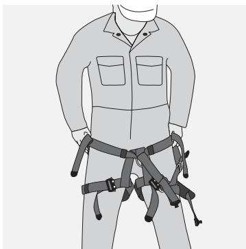
Pull the harness upwards to waist level
