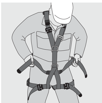
Tighten waist strap by pulling both sides
