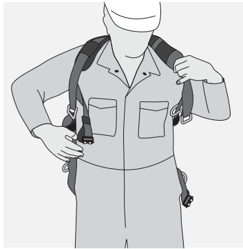
Place both shoulder straps over the shoulder as in donning a vest
