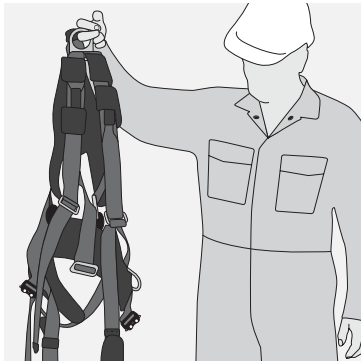
Hold harness by the Rear D with all straps undone
