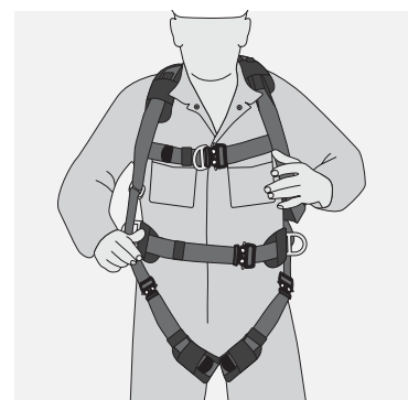
Fitted harness should be snug and firmly fitted, particularly the leg straps
