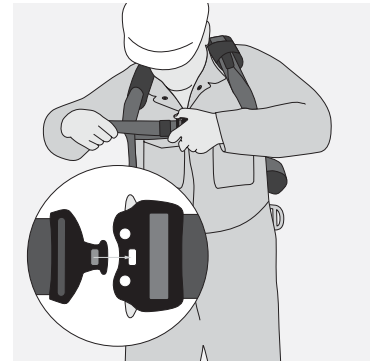
Connect chest buckle, ensuring that green spot is seen in the receiver window. Tighten strap.
