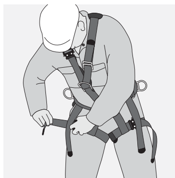
Tighten leg straps
