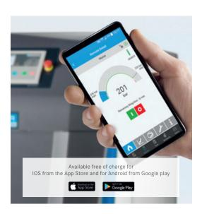
The new B-APP<sup>1</sup> communicates with your compressor system using WiFi. It provides simple, direct remote access to functions of your high-performance B-CONTROL MICRO compressor control unit.
