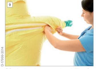
Slip the hood over your head. The air should noticeably flow over your back. Have the zipper and the cover flap on the back closed by another person.
