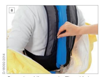
Open the airline supply. The whistle will sound briefly as the pressure increases. Open or close the zippers of the vest to regulate the cooling effect.
