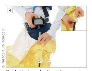
Guide the hose for the airline supply through the entry tunnel into the suit. Connect the airline supply to the input coupling. Close and seal the tunnel by closing the hook-and-loop fastener tightly around the hose.
