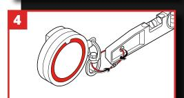
For the Auto-Stop unit, pass a Gripplock Cable or Screwlock Cable through the spare D-Ring and fasten the Cable.
