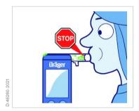
With a non-return valve, the intake of potentially contaminated air is not possible.
