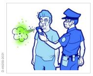
When the sample is taken, the air flows past the device and there is a 90 degree angle between the operator and and the test subject possible.
