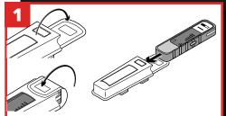
Ensure Radman or electronic device has a GRIPPS® E-Catch applied. Open top cover and slide Radman/device all the way to the bottom of holster. Close top cover after.
