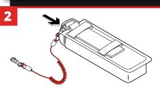
Connect a GRIPPS® Poly Clip to the D-Ring at top of holster by pressing clip end into D-Ring.
